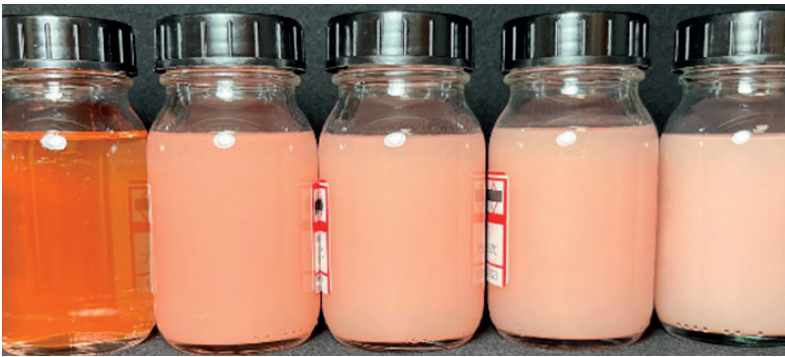
Without opacifier 2% in weight natural opacifier 3% in weight natural opacifier 4% in weight natural opacifier Styrene acrylate copolymer
