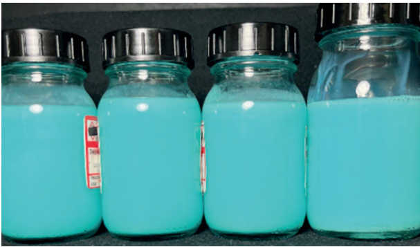
3% in weight natural opacifier 4% in weight natural opacifier 5% in weight natural opacifier Styrene acrylate copolymer
